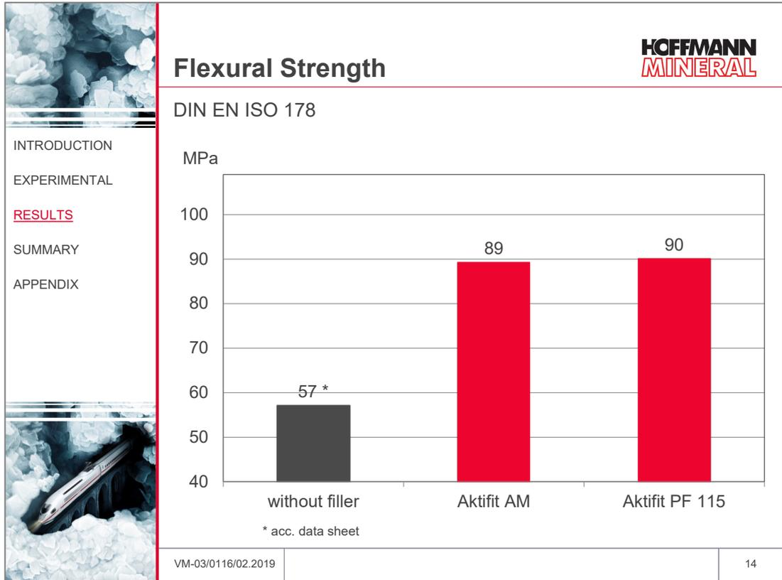
Also the flexural strength is significantly higher for the filled compounds than the unfilled compound, without having a noticeable difference between the two Neuburg Siliceous Earth fillers.
