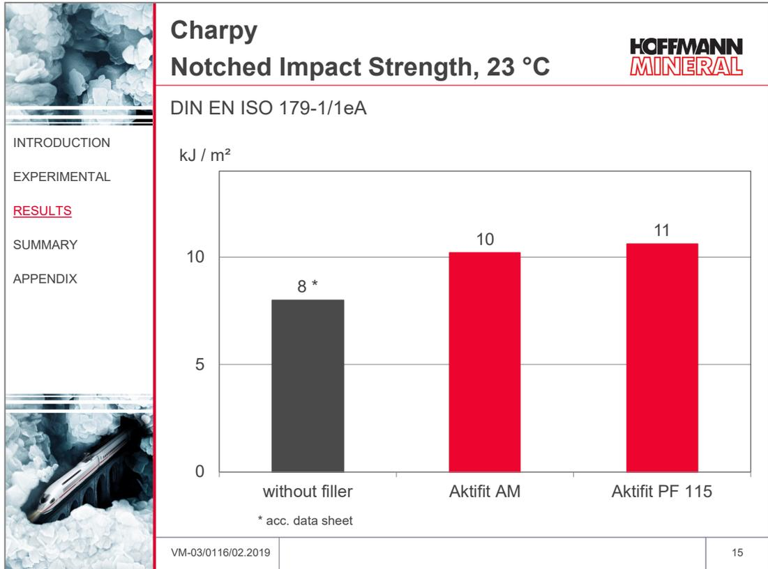
The notched impact strength will be increased by the addition of fillers from 8 kJ/m<sup>2</sup> to 10 kJ/m<sup>2</sup>.
