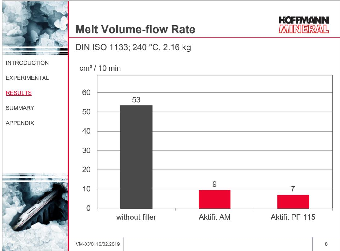
The filler-loaded compounds exhibit a markedly lower volume-flow rate compared with the unfilled polymer. However, they can be extruded without giving rise to premature crosslinking problems.
