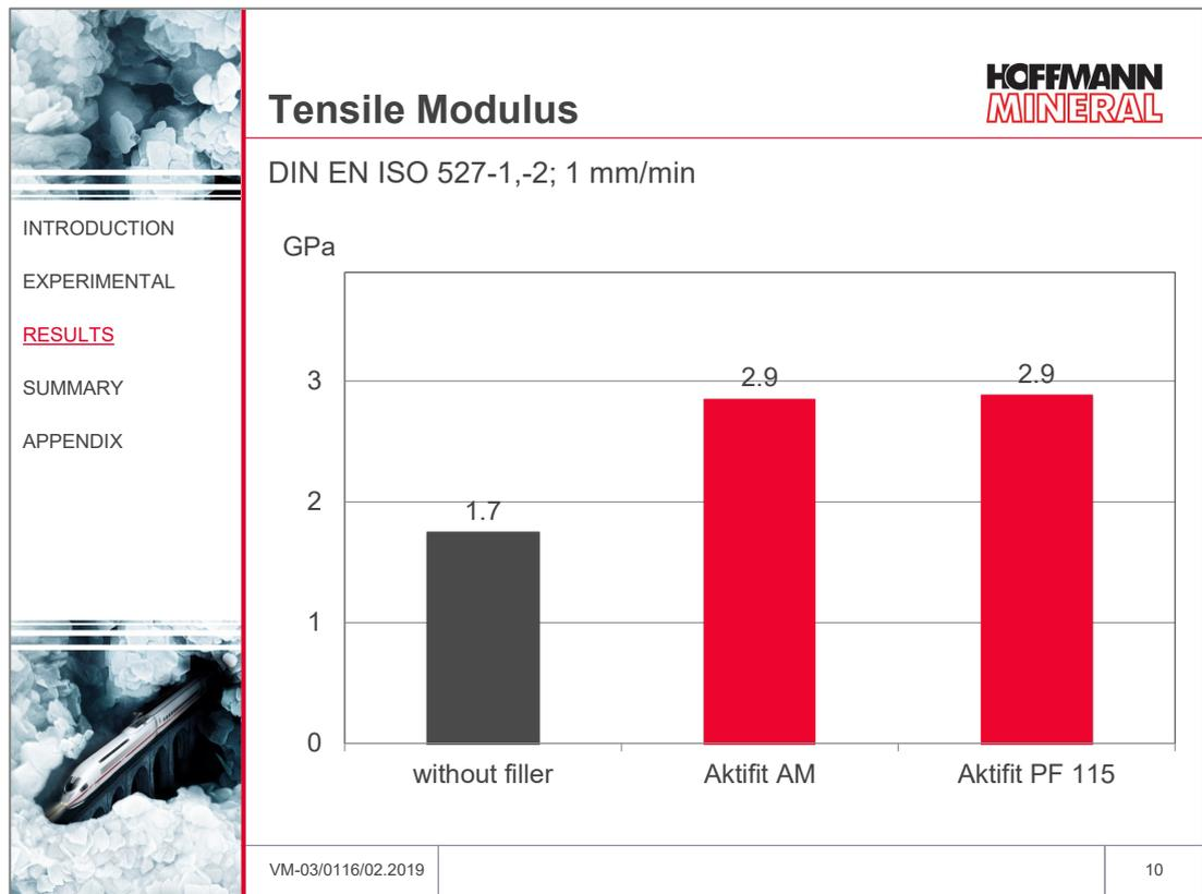
The compounds loaded with the Siliceous Earth grades, according to expectations, exhibit a stiffness higher by 70 % in comparison with the unfilled polymer.
