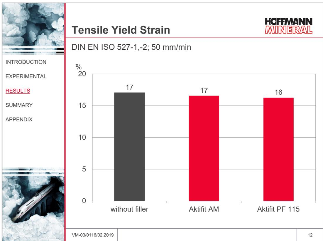
With respect to yield strain, there arise no negative effects of the mineral fillers, as the two compounds loaded with Neuburg Siliceous Earth grades show the same yield strain as the unfilled polymer.
