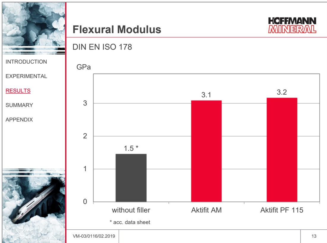
The unfilled polymer has with 1.5 GPa a significantly lower stiffness than the two filled compounds. Between the two Neuburg Siliceous Earth fillers, no remarkable difference can be noted. The flexural stiffness comes off slightly higher than the stiffness of 2.9 GPa obtained in the tensile test, and thus the resulting increase tends to be somewhat above the 70 % increase of the tensile modulus.
