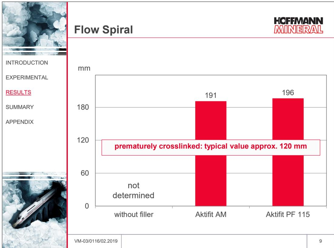
The flow path obtained gives an indication of whether or not a compound already starts to crosslink during extrusion. Typical results for prematurely crosslinking compounds with the mold in use are >120 mm. The flow distances with the two Neuburg Siliceous Earth grades of around 190 mm underline that the compounds can be extruded satisfactorily and without premature crosslinking.
