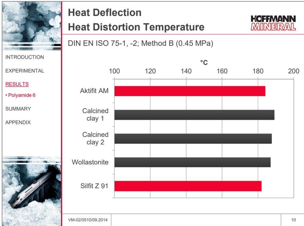
With the competitive fillers the heat deflection was marginally higher than with Aktifit AM, which can probably be explained by slight differences in the E- moduli.
