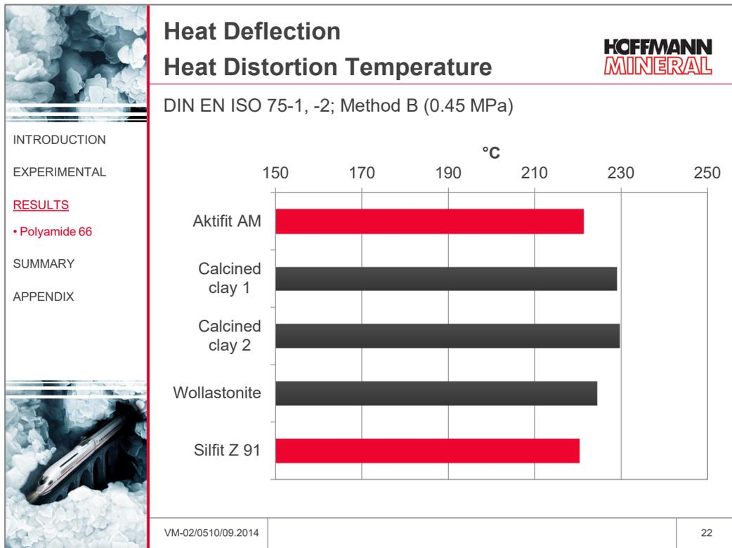
Both clays here give rise to a slightly higher HDT compared with wollastonite and Aktifit AM, which could be explained mainly by the somewhat different E-moduli.
