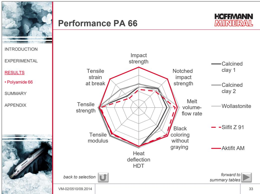
In the two polyamide 66 grades tested (Ultramid® A3K and Schulamid® 66 MV 2), Aktifit AM offered remarkable benefits with respect to impact strength and strain at break. Compared to the two calcined clays, better flow properties were evident, furthermore in black-colored compounds Aktifit AM made possible a deeper color without graying.
