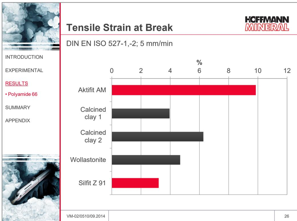
The breakage of the samples loaded with Aktifit AM occurred only at twice the strain of the competitive fillers. This represents an improvement of at least 50 % vs. the clays, and more than 100 % vs. Wollastonite. This effect should be of advantage for all applications where during assembly the components have to withstand certain deformations, such as in snap-fit connections.
