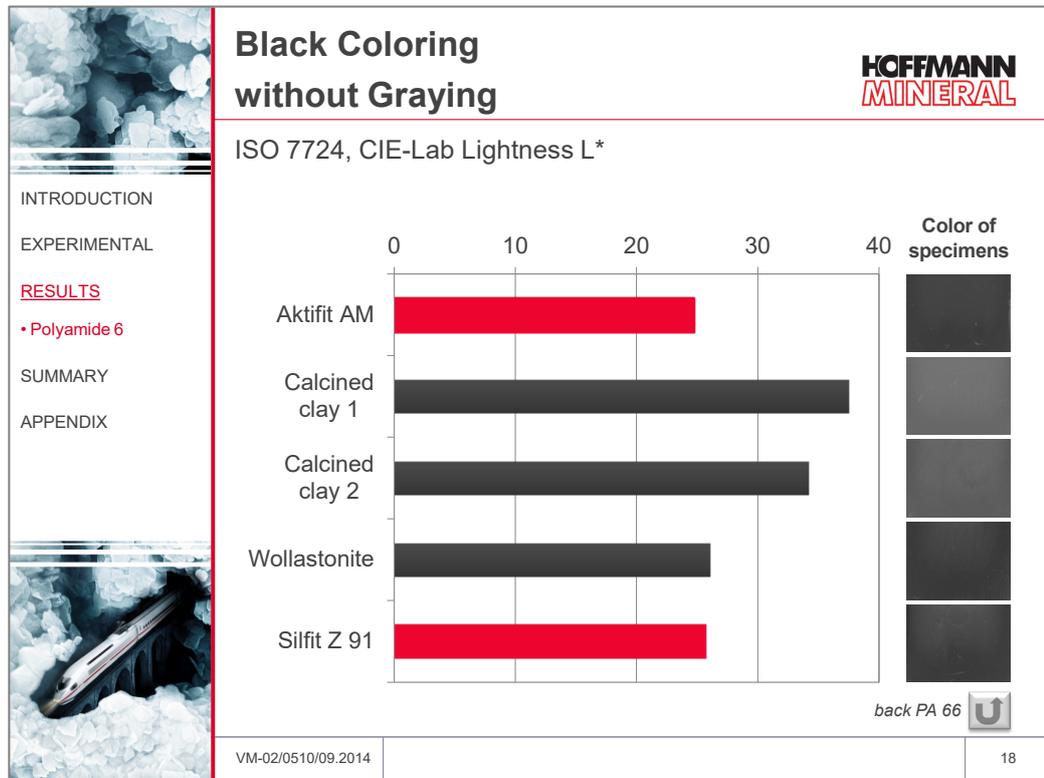
In the black compounds, the two clays give rise to a distinct brightening resp. grey coloring. With Aktifit AM, Silfit 91 and wollastonite this was not the case. As a multitude of polyamide applications is based on black-colored parts, avoiding of grey tones or a lower need for pigment batch with Aktifit AM represent an additional benefit.
