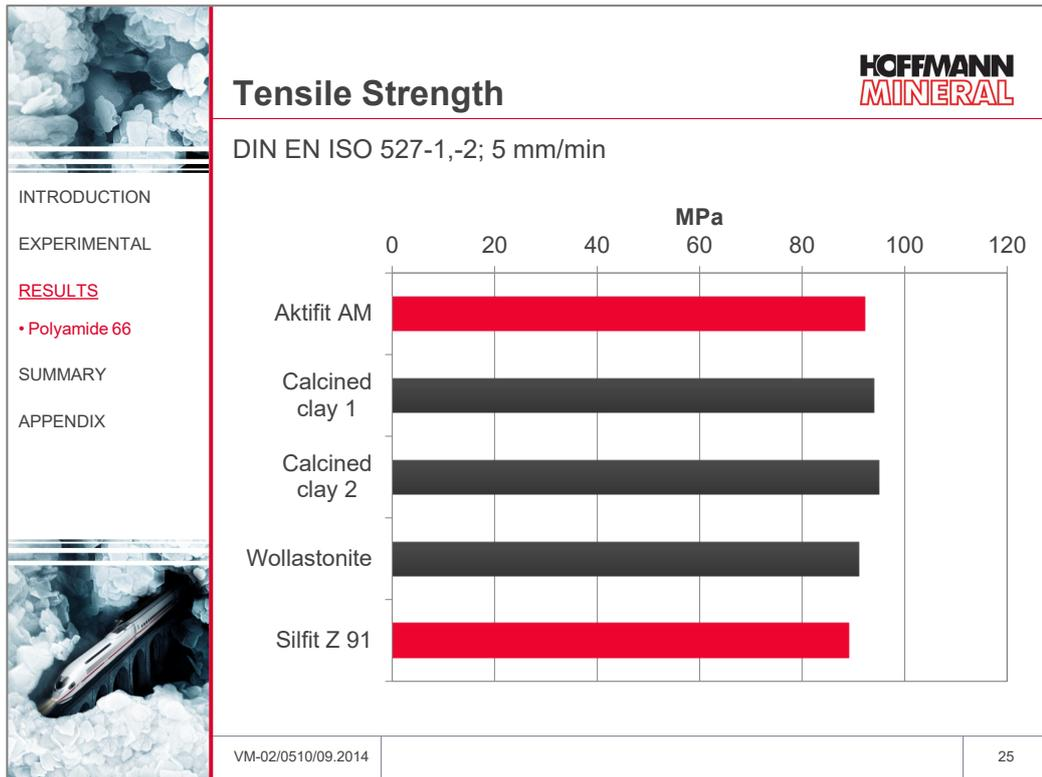
In the tensile tests, no significant differences were found for the tensile strength. The two clays tended towards marginally higher results.
