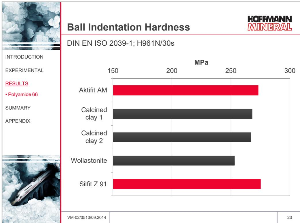
The ball indentation hardness with the calcined Neuburg Siliceous Earth grades was found at a higher level vs. the competitive fillers, especially wollastonite.
