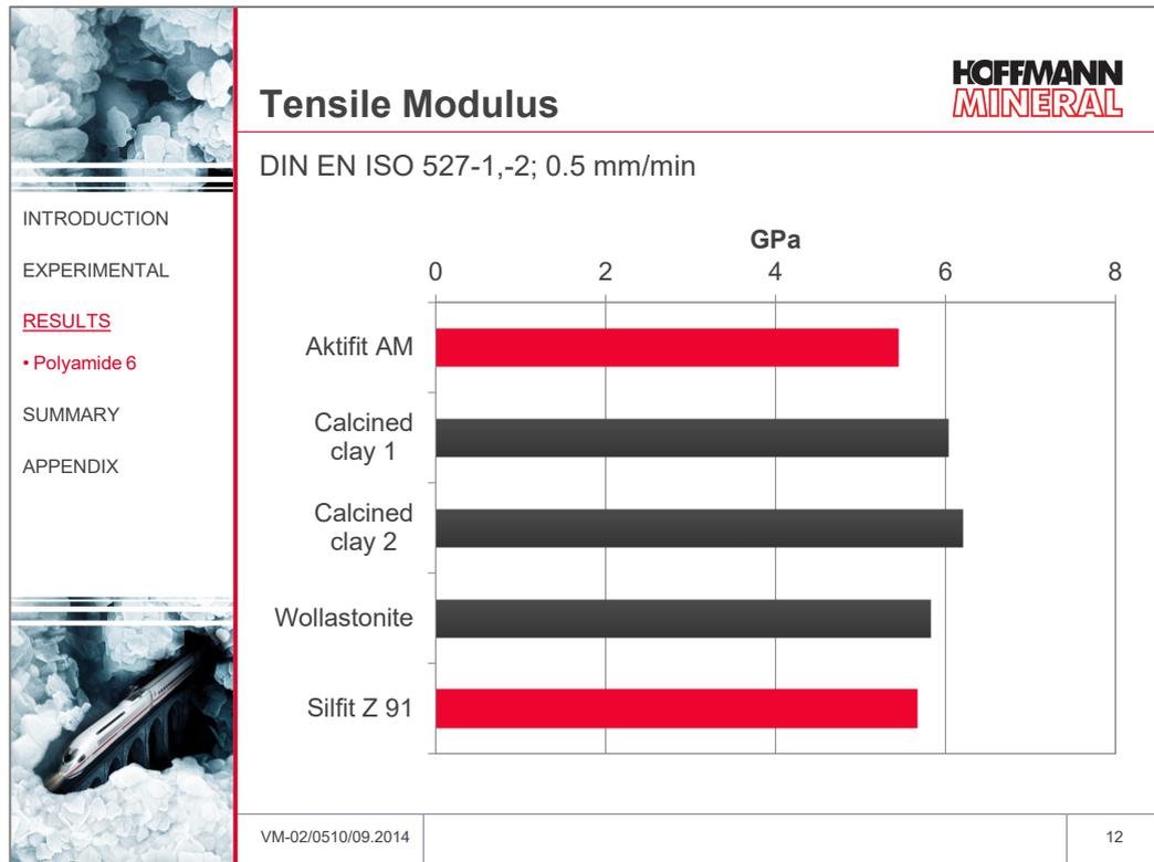
With the two clays, especially clay no. 2, the stiffness was somewhat higher. Aktifit AM arrived at a level almost similar to wollastonite.
