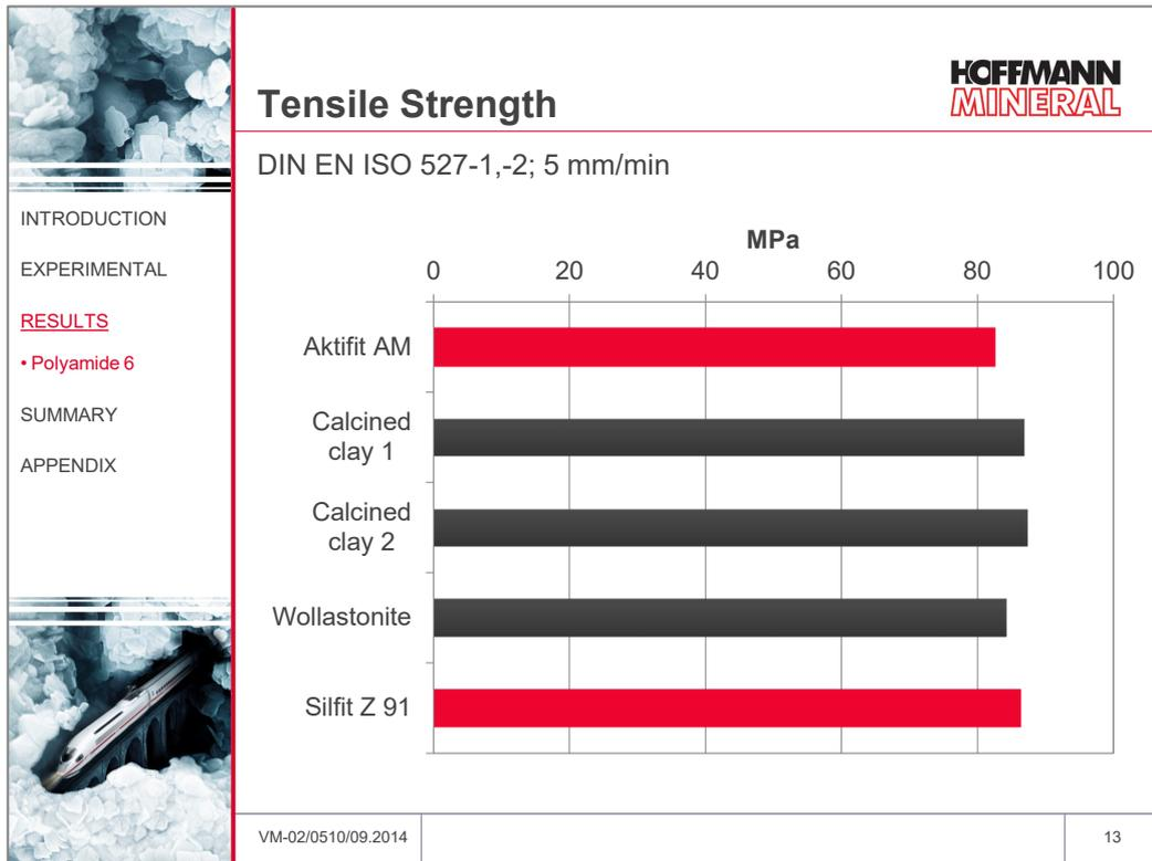
The tensile test did not show any noticeable differences in tensile strength. Both clays had a tendency towards slightly higher results.
