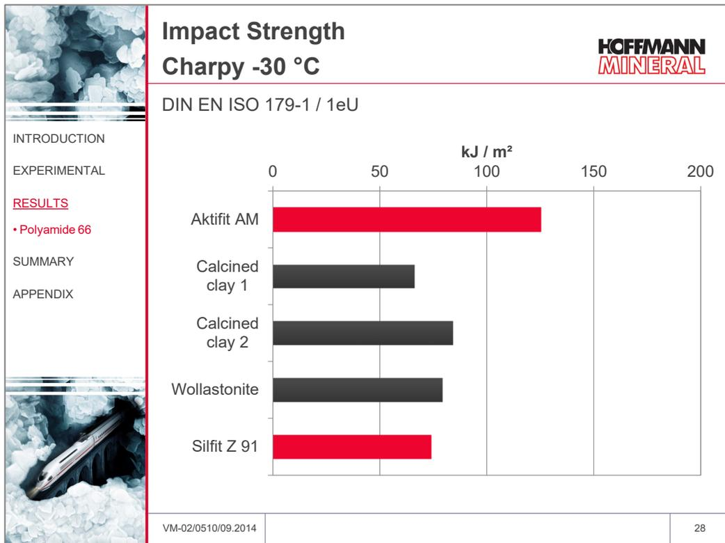
When tested at low-temperature, the overall level of the results decreased, but the ranking of the fillers and the significant advantage of Aktifit AM were maintained. At -30 °C the impact strength of Aktifit AM was even higher than with the other fillers at room temperature.
