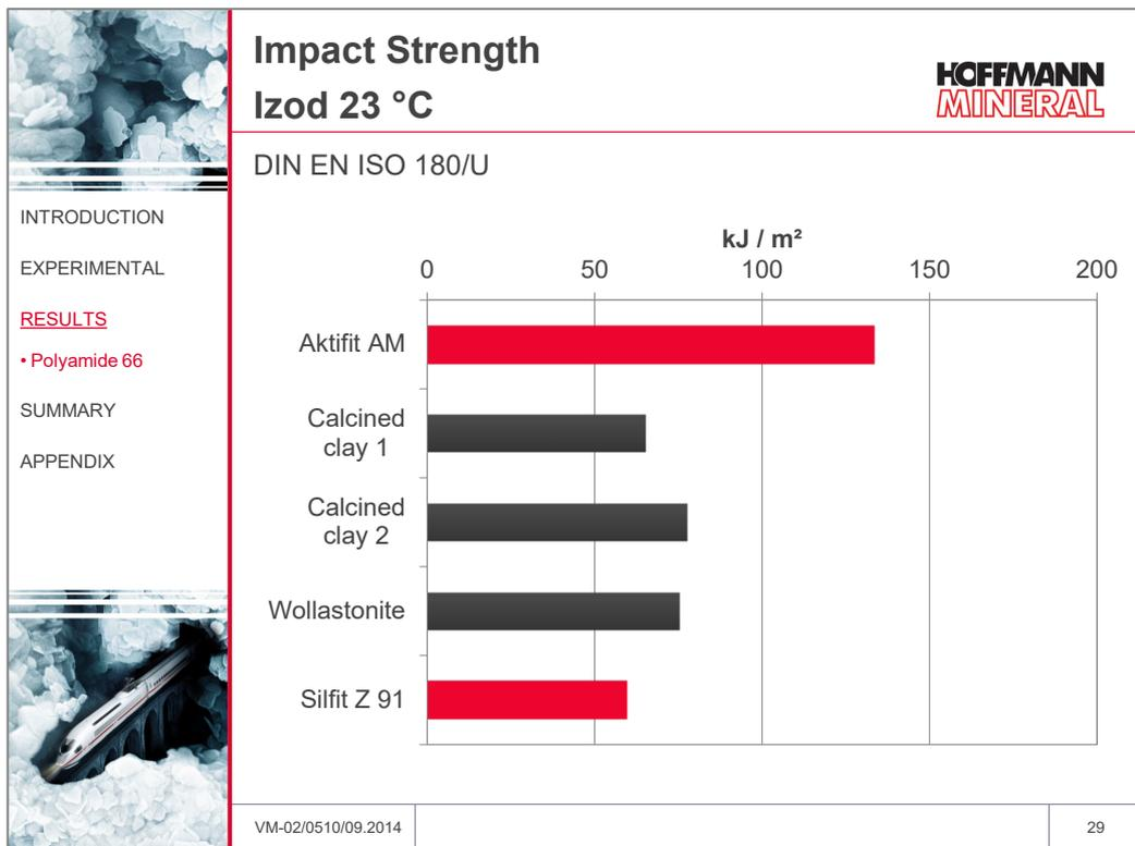
With Polyamide 66 too the different test arrangement according to Izod resulted in overall lower impact strength results. The ranking of the fillers, however, again remained the same.
