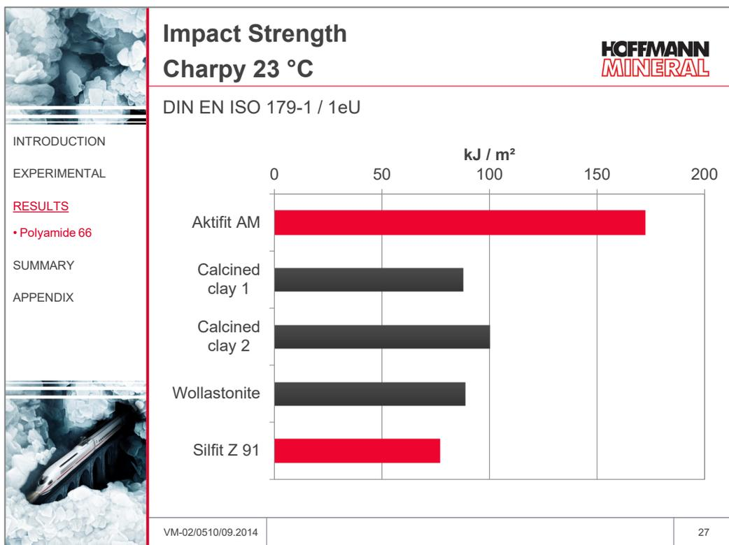
Aktifit AM, with an increase of up to 90 %, showed an impressively high Charpy impact strength, and thus marked advantages vs. the competitive fillers.
