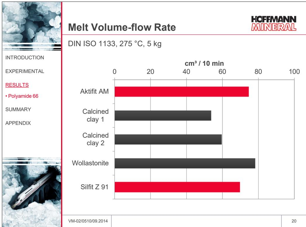
Aktifit AM in polyamide 66 gave similar flow properties to wollastonite, and therefore came out markedly better than the clays tested.
