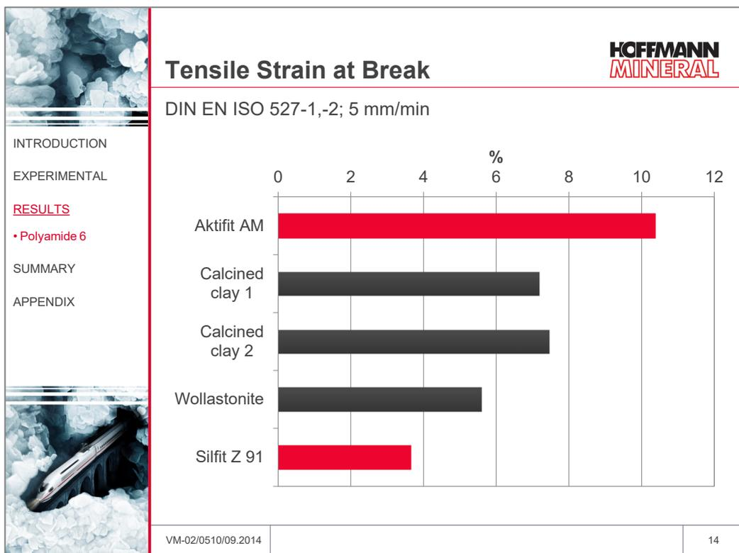
Compared with the competitive fillers, the samples with Aktifit AM suffered breakage only at a markedly higher elongation. The results corresponded to an improvement of 40 % vs. the clays, and 85 % vs. wollastonite. This effect should prove useful in applications where the components during assembly have to withstand defined deformations, such as snap-fit connections.
