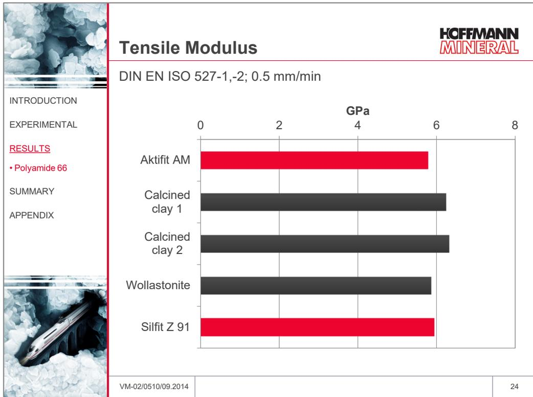
Both clays showed a somewhat higher stiffness. Aktifit AM came up to a level comparable with wollastonite.
