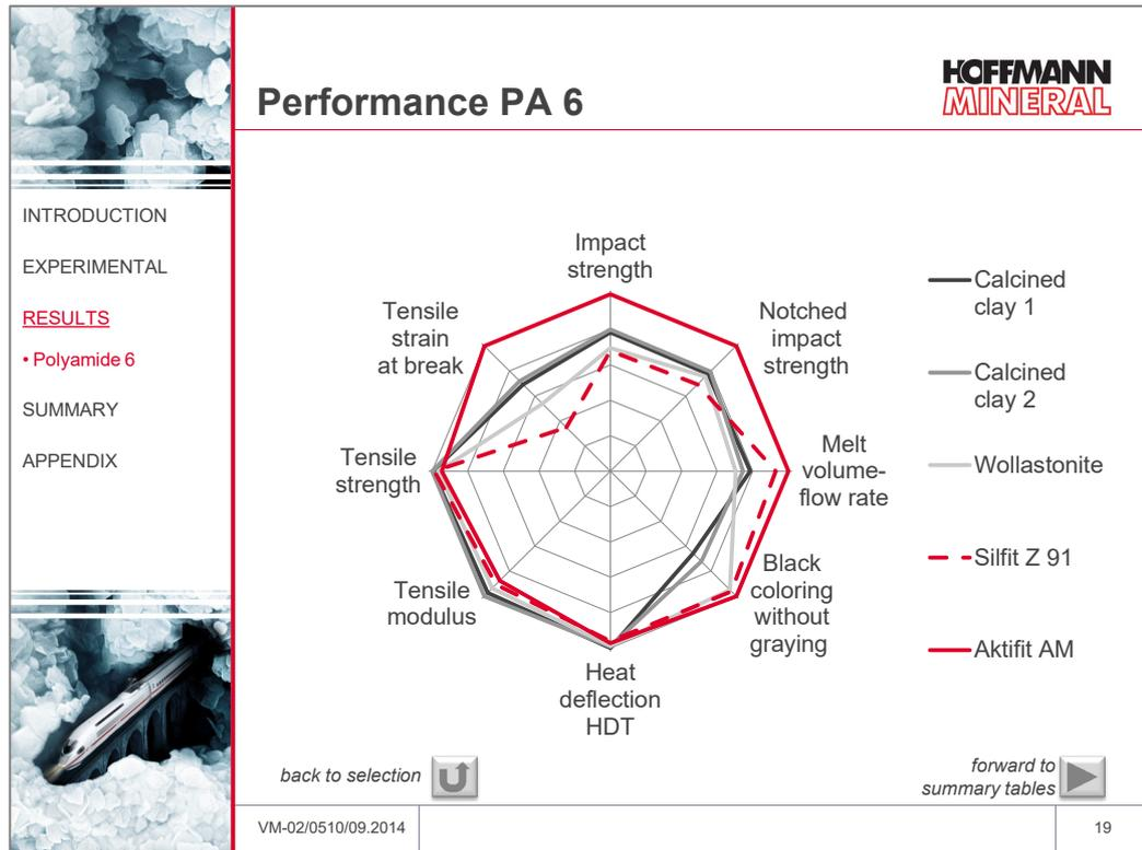
In polyamide 6, Aktifit AM was able to convince particularly with regard to impact strength and strain at break. In comparison with the calcined clays tested, the flow properties were distinctly improved. Black colored compounds could be prepared with Aktifit AM without brightening or graying. The tensile strength was maintained on the level of wollastonite. Marginal setbacks existed only with respect to the stiffness (tensile modulus).
