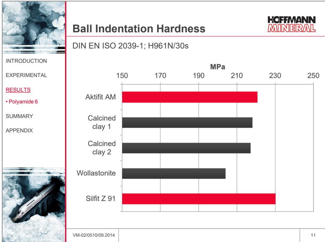
Calcined Neuburg Siliceous Earth gave rise to a higher hardness compared with the competitors, especially wollastonite.
