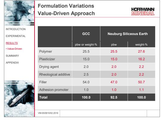
The table shows the base formulation with ground calcium carbonate and the formulation version adjusted for Neuburg Siliceous Earth with reduced filler and silica content. Among the Neuburg Siliceous Earth grades, Sillitin V 85, Silfit Z 91 and Aktisil VM are included.
