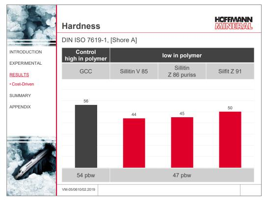
With the modified polymer/plasticizer ratio and reduced filler content, the hardness drops below the level of the polymer-rich base formulation with GCC. The use of the calcined grade Silfit Z 91 makes it possible to compensate this effect to some extent.
