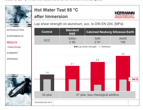
For the hot water resistance, the positive results with the Neuburg Siliceous Earth grades have been confirmed.
