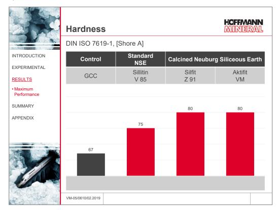
In the formulations without plasticizer, Neuburg Siliceous Earth grades result in a marked increase of the Shore hardness, which is most pronounced with the calcined products.
