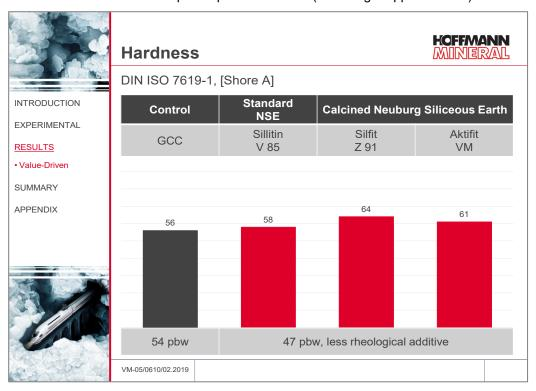
Calcined Neuburg Siliceous Earth – despite reduced filler content – produces a hardness increase.
