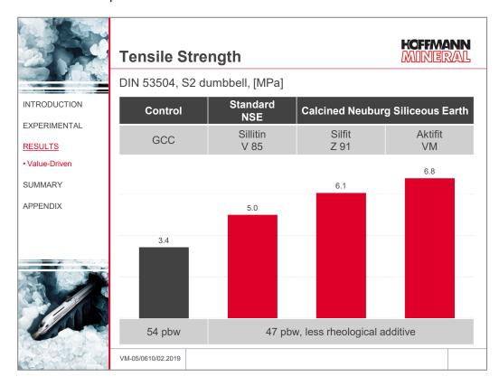
Despite the somewhat lower filler loading, Neuburg Siliceous Earth is able to impart a significantly increased tensile strength. Already Sillitin V 85, the coarsest and highly cost effective grade, brings about a marked improvement. With the calcined grades, the tensile strength in comparison to calcium carbonate can partly even be increased by a factor of two.
