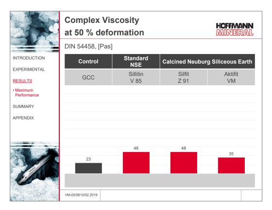
Under higher deformation the complex viscosity with Neuburg Siliceous Earth in direct comparison is higher than with GCC. Within the Neuburg Siliceous Earth grades, this increase turns out lower with the surface treated calcined grades.
