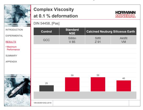
At low deformation, the Neuburg Siliceous Earth grades result in only marginally higher measuring values. Also under quasi-static conditions the batches give evidence of a pronounced flow tendency.
