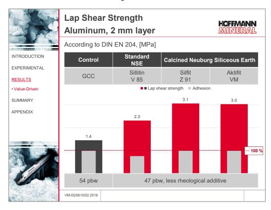
The Neuburg Siliceous Earth grades here again come off significantly better than the calcium carbonate. In particular, Silfit Z 91 and Aktifit VM give rise to an improvement of the lap shear strength of 120 %.
