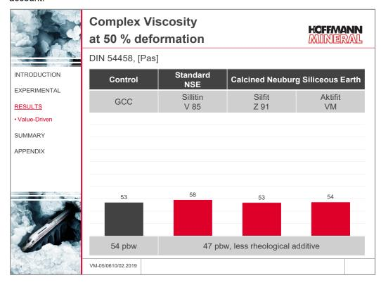
All formulations come up with about the same low complex viscosity at larger deformations. For application purposes, this means that all batches are extruded with similar ease as the formulation with GCC.
