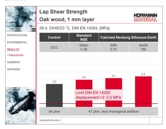
The standard DIN EN 14293 for "soft" parquet adhesives – as defined by a displacement above 2 at an adhesive layer thickness of 1 mm – calls for a lap shear strength of at least 0.5 MPa. This minimum requirement is easily exceeded without problems by all tested formulation variants. All batches gave evidence of good adhesion on the oak wood substrate. The product variants with Neuburg Siliceous Earth distinctly enhance the tensile level with an improvement of up to 33 %.
