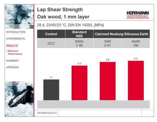
Despite very good adhesion, the extremely high tensile strength cannot fully be transferred to the substrate, yet compared with calcium carbonate the lap shear strength is still increased by a factor of 2 – in particular with the calcined grades. With this, the inherent strength of the oak wood is attained, so that partly wood fiber break-outs can be observed.
