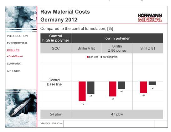
With respect to cost savings, the area of "soft parquet adhesives", as a result of the strength obtained with Neuburg Siliceous Earth grades, offers several chances. With a savings potential of 10 % (based on volume) resp. 7 % (based on weight), the formulation with Sillitin V 85 comes out as the most cost favorable choice.
