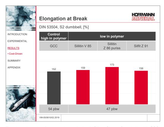
The elongation at break too remains on the level of the reference formulation with GCC. Sillitin Z 86 puriss shows a tendency towards higher elongation.
