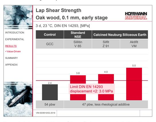
Here again the batches with Neuburg Siliceous Earth come out markedly higher than the minimum requirements, whereas with GCC also this limit cannot be overcome.
