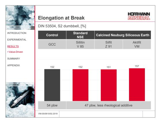
While the tensile strength is markedly increased with Neuburg Siliceous Earth, the elongation at break at the same time remains at the level of the base formulation with GCC. The reinforcing potential of Neuburg Siliceous Earth comes out in a markedly higher energy absorption capacity up to break, which can be determined as the integral of the stress over the strain (elongation).
