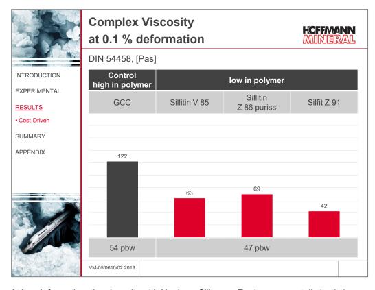
At low deformation, the viscosity with Neuburg Siliceous Earth comes out distinctly lower, and the flow tendency stronger. This is particularly true for the calcined Silfit Z 91. These trends could well be counteracted by proper adjustment of the filler and rheological additive loading, if higher non-sag is desired.
