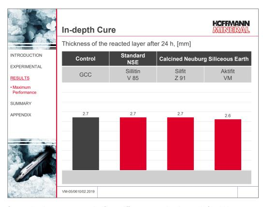
Concerning the cure rate, no significant differences can be observed after 24 hours.
