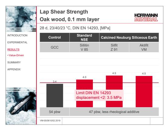
For "hard" adhesives – defined by a displacement below 2 – the standard specifies a lap shear strength of at least 3.5 MPa after 28 days of curing. Contrary to the control formulation with GCC, which just misses the limit, the batches with Neuburg Siliceous Earth have no problem in meeting this requirement. In so doing, the calcined siliceous earth grades give the best results.
