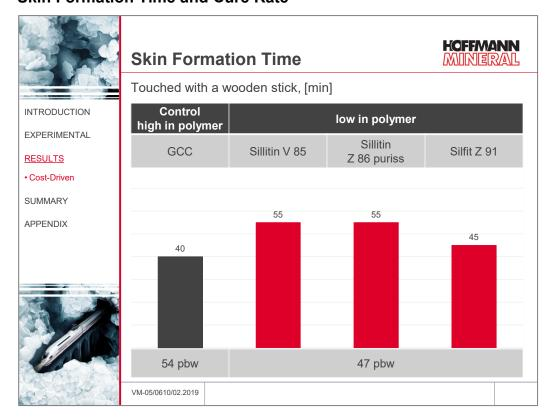
Compared with the polymer-rich formulation with GCC, the skin formation time is generally prolongated as a result of the increase in plasticizer content. This means a longer open time is available for placing the parquet. In particular the standard Siliceous Earth grades Sillitin V 85 and Sillitin Z 86 puriss offer themselves for use of this effect. When working with Silfit Z 91, the skin formation takes place at a similar rate as with the base formulation.
