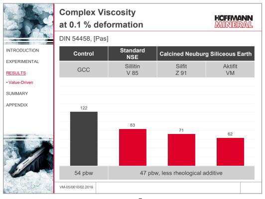
The Neuburg Siliceous Earth grades at low deformation give a lower complex viscosity than the calcium carbonate. This indicates a stronger flow tendency, which is, however, easily compensated by increasing the silica addition to 2.5 to 3 parts by weight.
