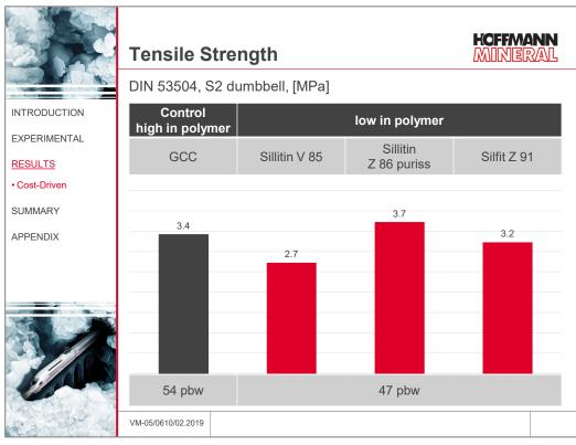
With the finer particle size of the Siliceous Earth grades Sillitin Z 86 puriss and Silfit Z 91, the tensile strength rather remains at the level of the polymer-rich reference with GCC. The coarser grade Sillitin V 85 leads to a slight loss.
