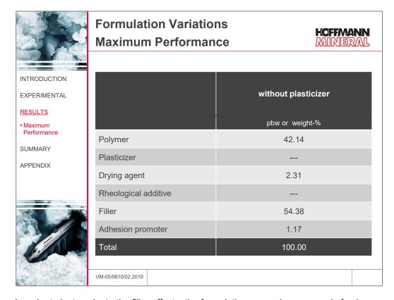
In order to just evaluate the filler effects, the formulation was only composed of polymer, filler, drying agent and adhesion promoter. The rheological additive was left out, due to it also contributes to the strength, and additionally tends to increase the viscosity.
