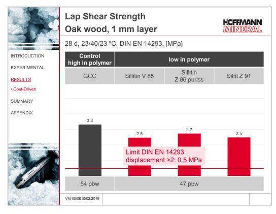
The lap shear strength admittedly is somewhat lower compared with the polymer-rich GCC formulation, but still goes much beyond the requirement of DIN EN 14293 for "soft" adhesives. All formulations give evidence of good adhesion to the oak wood substrate.
