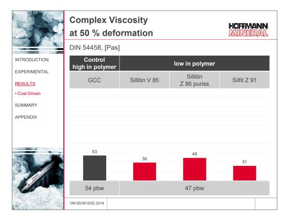
Caused by the reduced filler content and the inverted polymer/filler ratio, the formulations with Neuburg Siliceous Earth at larger deformation show a lower, at maximum comparable viscosity level compared to the base formulation with GCC.
