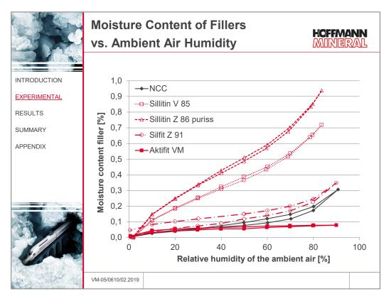
The curves refer to the moisture uptake with increasing humidity of the surrounding air, as well as the moisture loss with decreasing humidity of the ambient air.
