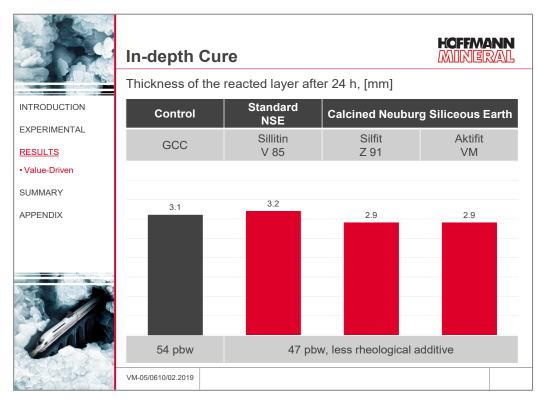
While Sillitin V 85 imparts a similar cure rate as GCC, the thickness of the reacted layer with the Calcined Siliceous Earth grades comes out somewhat lower. The results, however, are always close to each other, so the minimum differences should not be overestimated.
