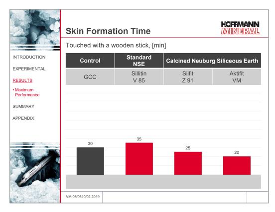
The formulation with the standard grade Sillitin V 85 requires a marginally longer time for skin formation. With the Calcined Siliceous Earth grades – especially with the surface treated product – the skin formation time comes out somewhat shorter.
