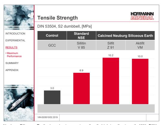
Neuburg Siliceous Earth gives rise to an extraordinarily high tensile strength. With Sillitin V 85, the tensile strength can already be more than doubled vs. GCC. Silfit Z 91 and Aktifit VM with approx. 10 MPa give the very best results, which is more than three times the level of the GCC formulation.
