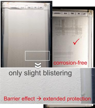
only slight blistering<br>corrosion-free<br>Barrier effect → extended protection |
