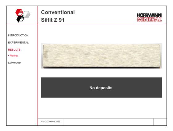
As evident from the figure, with Silfit Z 91 no deposits can be spotted on the metal insert. The visual evaluation at 100x magnification confirms this result.
