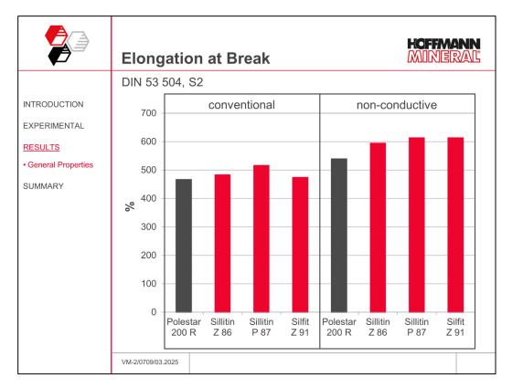
As shown in the graph, in the conventional compounds the highest elongation at break is obtained with Sillitin P 87; Silfit Z 91, Sillitin Z 86 and the calcined clay come out at a somewhat lower level.
