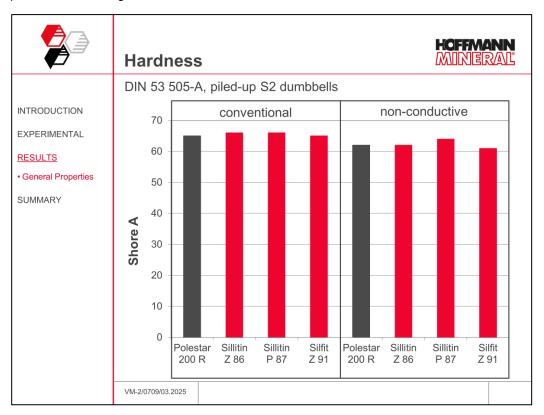
Hardness was determined on three piled-up S2 dumbbells. No significant difference can be found between the individual fillers.
