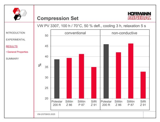
The test conditions for the compression set according to the VW test standard 3307 were 70 hours at 100  $^{\circ}$ C under 50 % deflection, cooling down for 3 hours (still under deflection), and a relaxation time of 5 seconds .
