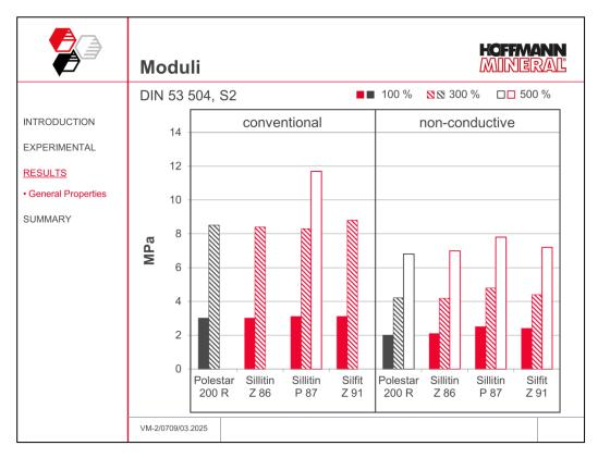
The moduli obtained with the individual fillers are on a comparable level, both for the conventional and for the non-conductive formulations. The partial replacement of carbon black in the non-conductive compounds results for all formulations in a lower level of the moduli compared with the conventional approach.
