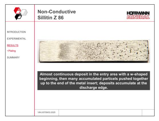
With Sillitin Z 86 in the electrically non-conductive compound, a continuous deposit is formed at the entry area with a w-shaped onset. After that, many pushed-together particle accumulations are visible up to the end of the metal insert, which gather close together at the exit edge. Deposits can be seen on the surface opposite the metal insert, too. The visual assessment at 100x magnification confirms this result. Sillitin P 87 shows similar characteristics.
