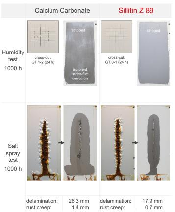
Cold rolled steel Q-Panel R 48, spray application, total dry film thickness 70 µm as single-layer, drying 28 d 23 °C / 50 % RH
